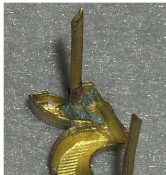
Larger TR devices usually had soldered on flat prongs with angle cut ends
